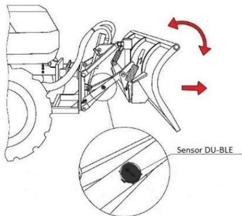
Fig.6. Installation of the DU-BLE on plow-type devices
