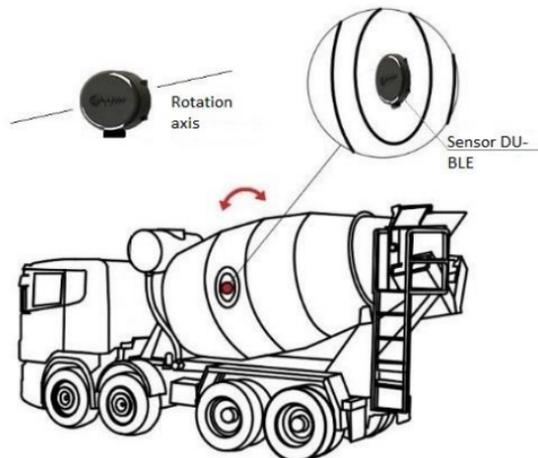
Fig. 2 Installation of the DU-BLE on the cement-mixer in vertical rotation control mode.
